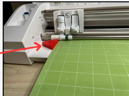
While holding the mat, press **load** on the screen of the machine.
