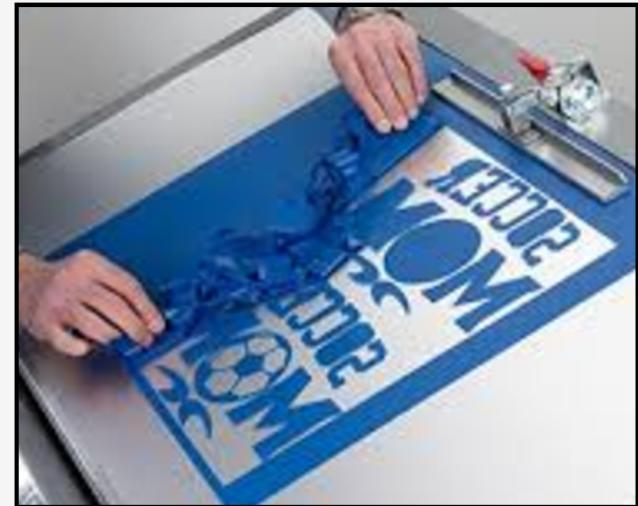
With heat transfer vinyl, you are now ready to heat press your design onto your material! Set the press for 315 degrees and 15 seconds.
